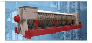
The **Dupps Stickwater Evaporator** features falling film technology that minimizes liquid retention time, reducing product degradation as well as waste during cleaning. Available as a single or multiple effect system, it can be designed to use waste process vapor and/or high pressure steam as a heat source. ASME Code design and stamping is available, as is an automatic, tube side clean-in-place system.
