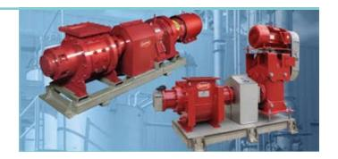
Dupps Fish Cookors™ feature a unique shaft design that promotes uniform temperature throughout the cooking zone for a more consistent, high-quality product. It also enhances oil, water and solids separation downstream of the cooker. The shell and shaft are indirect steam heated — indirect steam can be returned to the boiler without treatment, and no direct steam injection means less evaporation load on the entire system.
